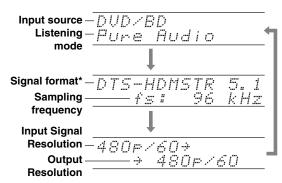
\* If the input signal is analog, no format information is displayed. If the input signal is PCM, the sampling frequency is displayed. If the input signal is digital but not PCM, the signal format and the number of channels is displayed. For some digital input signals, including multichannel PCM, the signal format, number of channels, and sampling frequency is displayed.
